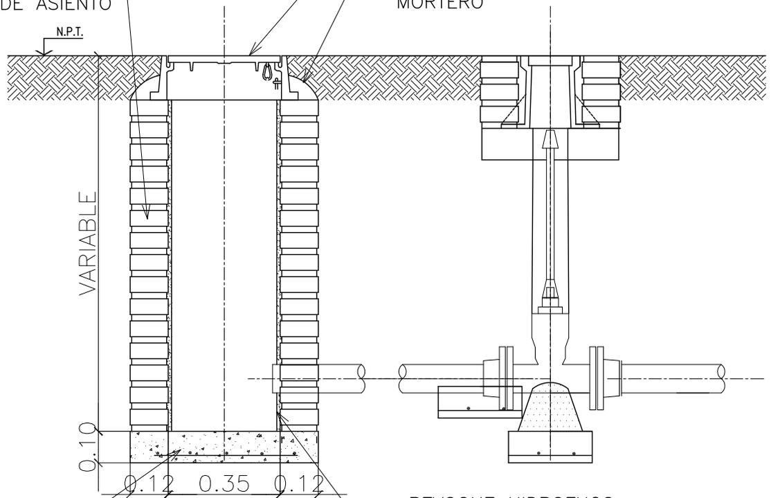
LOSA INFERIOR HORMIGON TIPO H-21 ACERO ADN-420  $\phi$ 10 c/15
